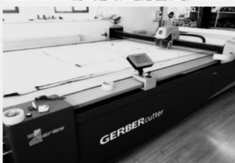
3 Axis CNC: Fabric and Leather cutter
